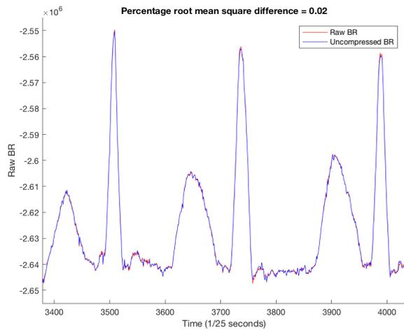
As for ECG, breathing compression and decompression preserve the most prominent features of the signal and smooths out high frequency noise.
