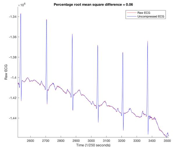
Here we show the result of the original ECG signal in red superimposed with the corresponding decompressed signal in blue. If the PRD was 0 (perfect decompression) then we would see only blue as it would perfectly superimpose the red signal. So we can thus see in red where the algo makes mistakes. The errors are mostly from smoothing very high frequency but low amplitude noise along the signal, there is no distortion in the most prominent signal features of the PQRST complex.
