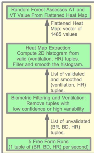
Fig. 2: Flowchart for assessing an AT and a VT from the system. The input is Breathing Rate (BR), Breathing Depth (BD), and Heart Rate (HR), as well as the number of RR intervals, for every second of each of the five runs. Tuples with low confidence or high variability are removed by the biometric filter, breathing variables are smoothed, and the ventilation is computed. The heat map is computed, which then provides a fixed size representation to the random forest model.
