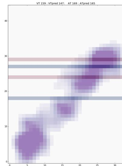
Fig. 4: Example heat map. Ventilation along x-axis, heart rate along y-axis. Demonstrates one form of ambiguity that can occur: there is not clear VT inflection point. As a result the manual VT (lower red bar) and algorithmic VT (lower blue bar) are far apart.
