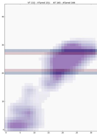
Fig. 3: Example heat map. Ventilation along x-axis, heart rate along y-axis. Demonstrates good inflection points obtained from free form run data. Manual (red bars) and algorithmic (blue bars) AT and VT values are very close.
